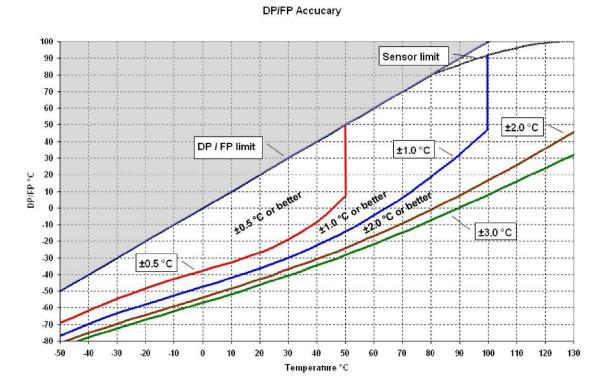
**Example**: at a temperature of 20 °C, a dew point value of -37 °C is measured with an accuracy of ±1.0 °C or better.
